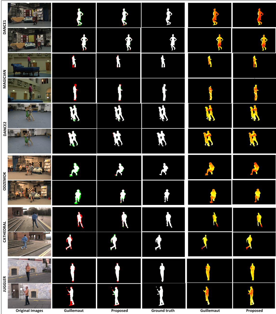
Figure 5. Results for a pair of images from each dataset: 2^{nd} - 4^{th} column: Segmentation (Red represents true negatives and green represents false positives compared to the ground truth) and 5^{th} - 6^{th} column: Depth
