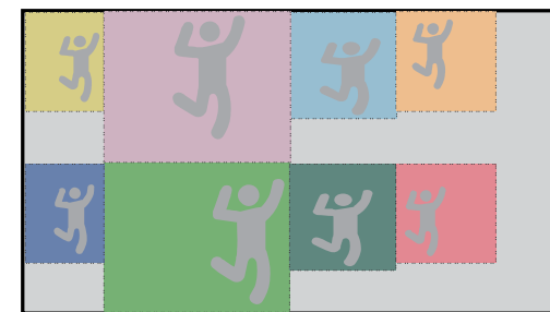
Packed ROI image for CPM detection (from frames B and C)
